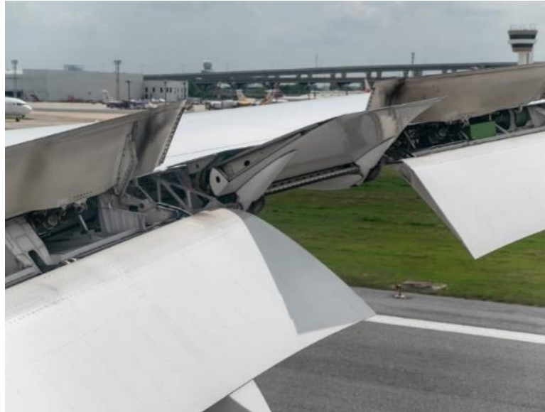
Fig 1. An Aircraft's Flap Assembly Consists of Complicated Sub-Systems and Parts (From Authors' Collection)
